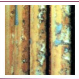
As a result of combustion and depending on the type of fuel and temperatures, vanadium, alkali metal sulphates and alumina silicates will form hard deposits
